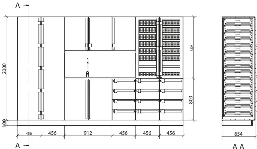
**Standard enclosure width 456 mm, depth 654 mm**
