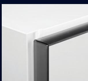
Doors and drawer fronts are made from 16 mm chipboard with 0.7 mm laminate to both the front and back. Edges are sealed with impact resistant and 2.0 mm 3D alloy/synthetic lipping for optimal hygiene.
