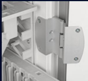
Zystm's cabinet hinge is specifically designed for hospital and laboratory use. The anodised aluminium quality hinge comes with self lubricating washers to the moving part. The hinge has been rigorously tested to 200,000 opening and closings with a maximum opening of 270 degrees.
