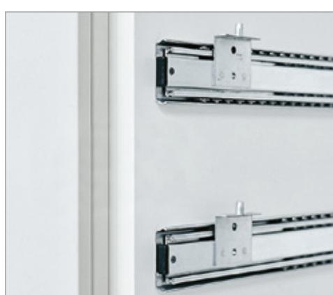
Telescopic slides are constructed from galvanised steel and corrosion protected. Precision pull-out on double ball bearings, ensuring a steady and smooth movement. The extension can be loaded with up to 60 kg.
