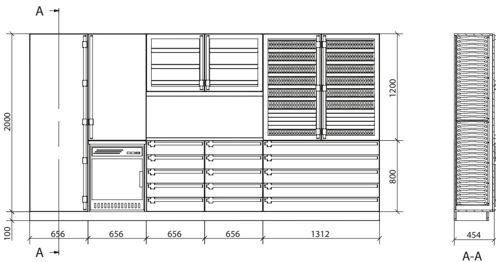
**Standard enclosure width 656 mm, depth 454 mm**
