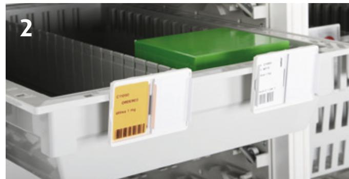
The contents of the left side of the tray is used. Left sign is slid to the right, new products are automatically ordered. The sign on the right side is activated by the left sign being slid to the right and the "Prohibited" sign removed. The contents on the right side can now be used.
