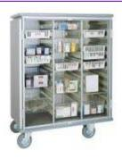
MODUL-iT container cart (ISO) in anodised aluminium with 3 sections for 3x12 pairs of plastic module rails in total. The 2 doors open 270° and can be fixed to the cart side with a magnet. The cart is surrounded by a bumper on both the upper and the bottom side, has 2 swivel wheels and 2 fixed wheels with ball bearing of Ø 16 cm. Dim. 140x71x178,5 cm (LxDxH)
