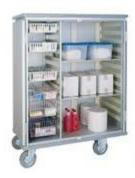
MODUL-iT container cart in anodised aluminium (ISO) with 1 module section for 12 pairs of plastic module rails and 1 section with two height-adjustable shelves of 85x60 cm (+ bottomshelf). The 2 doors open  $270^{\circ}$  and can be fixed to the cart side with a magnet. The cart is surrounded by a bumper on both the upper and the bottom side, has 2 swivel wheels and 2 fixed wheels with ball bearing of  $\emptyset$  16 cm. Dim. 140x71x178,5 cm (LxDxH)
