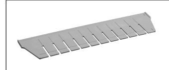
The teeth of the short dividers point downwards. These dividers must always be placed in the module after the long dividers. All short dividers can be shortened at the predetermined breaking points.
